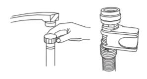
Connect the cold water supply hose to a threaded 3/4(inch) connector and make sure that it is fastened tightly in place.
