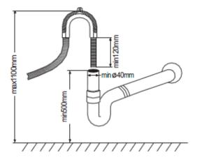
If the length of the hose is not sufficient, contact the authorized service supplier for an extension made from the same material as the original. Remember that the length of the hose should not exceed 4 meters even when with an extension.
